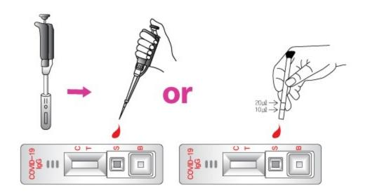
Add 10μℓ (serum or plasma) or 20μℓ (whole blood) of specimen into the sample well (S) using provided capillary pipette or micropipette.
