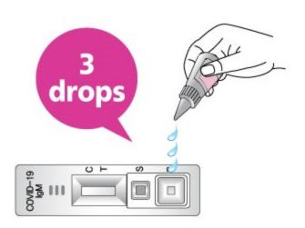
Add 3 drops of assay diluent into the buffer well (B) of the device.
