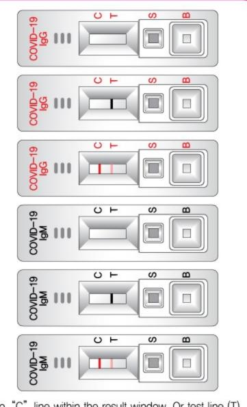
No "C" line within the result window, Or test line (T) appears in red faintly. It is recommended that the specimen be retested.
